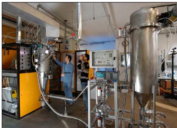
Fig. 5 Reactor prototype developed at the EMPA of Thun for the synthesis of nanoparticles (Ref 27)
